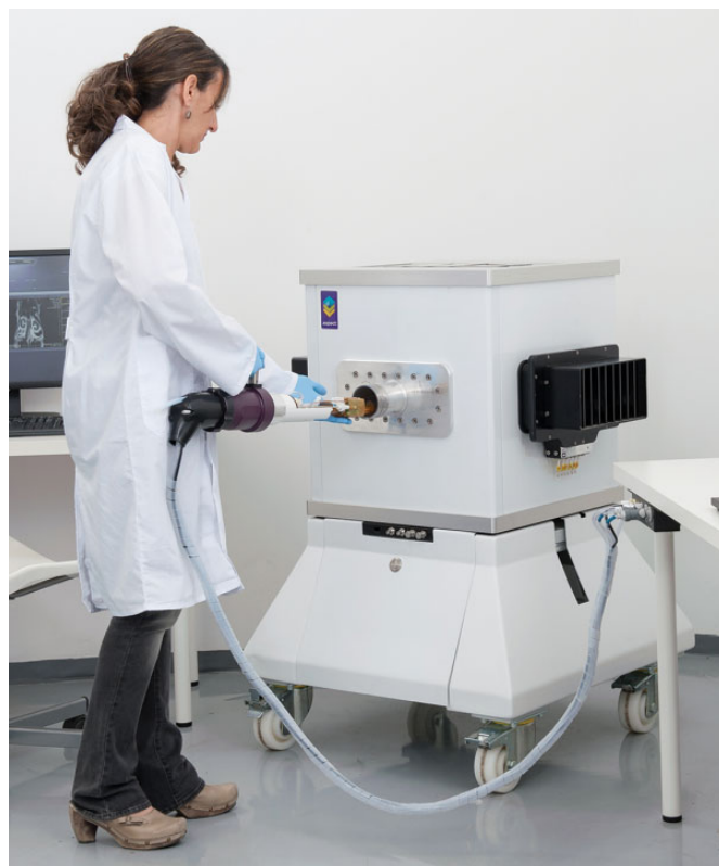
FIGURE 1.—Presentation of the new compact M2™ high-performance magnetic resonance imaging (MRI) platform for in vivo and ex vivo MRI-based histology applications (Aspect Imaging, Israel). The M2 system is a compact, high-performance MRI system that uses a permanent magnet, which ensures there is no external magnetic field enabling the system to be operated in most facilities and does not require any shielding, speciality facilities, or cooling and cryogenics to maintain the magnetic field. It is equipped with rat and mouse body and head coils. Animals are kept anesthetized with 2% isoflurane in O 2 on a specially designed heated bed and physiological signals are monitored throughout the experiment to ensure well-being of the animals. High-resolution ex vivo MRH is performed using a 20 mm radiofrequency (RF) coil on the same compact high-performance MRI system. In this configuration, the system allows high-throughput and automatic scanning of up to 10 samples without technician intervention. Briefly, fixed samples are introduced in specially designed disposable capsules that are given a unique bar code. The operator assigns predefined MR protocols to the bar coded sample, according to the organ or pathology under investigation. Up to 10 capsules can then be loaded into the system, which automatically advances, scans, and ejects the capsules one at a time. No intervention is required throughout the process, so samples can be left unattended to be scanned overnight.
